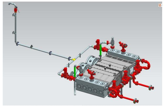
The Discharge Manifold will be an "H" type manifold, be rated 15,000 psi and will include 2" FIG 1502 Pipes, Fittings, Swivels and 2" x 2" Hydraulic Plug Valves.
